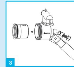
3 To access the diaphragm washer remove white plastic insert.
