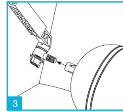
3 Fit suitable ball float to end of float arm. The position of the ball can be adjusted by loosening plastic wing nut, when desired position is achieved re-tighten wing nut.
