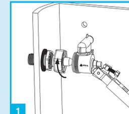
1 Ensure water is switched off and loosen the retaining nut.
