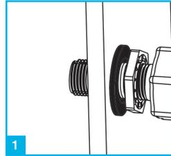
1 Remove the plastic washer and nut from the thread and position the valve in the cistern.
