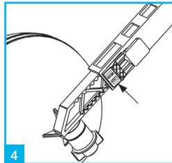
4 The arm length can also be adjusted by sliding the adjustment clip to unlock, move the arm in or out to desired length then lock the clip.
