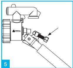
5 The water level can be adjusted by turning the adjustment screw (clockwise for less water, anticlockwise for more water).
