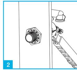
2 Secure valve to the cistern by replacing the plastic washer and screwing the nut to the thread. Do not over tighten.
