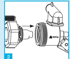
2 Remove the valve from the retaining nut.
