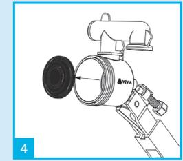
4 Remove the diaphragm washer and clean or replace.
