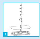
Remove spring and clip then replace the diaphragm washer.
