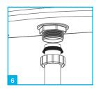
Low level installation does not require a close couple kit. Slide back nut and conical washer over the flush pipe and insert flushpipe into base of flush valve and secure with back nut
