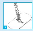
Once diaphragm washer has been replaced, secure clip and re-fit spring.
