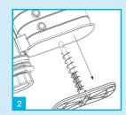
Slide stem through base to access the suction unit.
