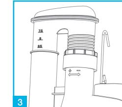
To adjust the height of flush valve twist the height adjustment screw and set to the desired height.
