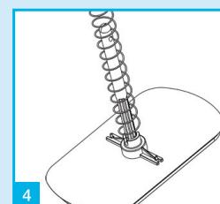
Once diaphragm washer has been replaced, secure clip and re-fit spring.
