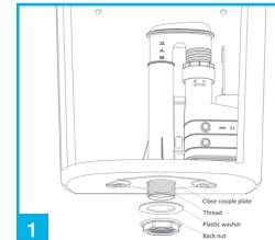
Insert the flush valve into the water tank. Slide close couple plate over siphon thread and tighten to the tank using the washer and nut.
