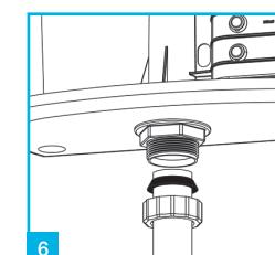
Low level installation does not require a close couple kit. Slide back nut and conical washer over the flush pipe and insert flushpipe into base of flush valve and secure with back nut.
