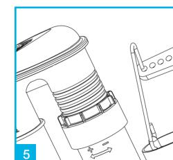
To operate flush valve connect the C-link to the toilet handle lever arm.
