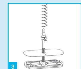
Remove spring and clip then replace the diaphragm washer.
