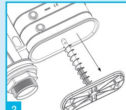
Slide stem through base to access the suction unit.
