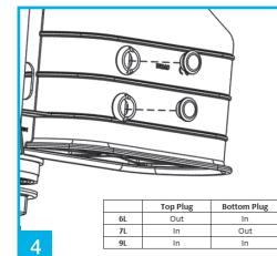
The flush volumes can be adjusted by removing the volume plugs. (Please refer to guide above)
