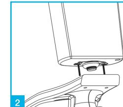
Fit doughnut washer and bolts and secure cistern to pan with wingnuts.
