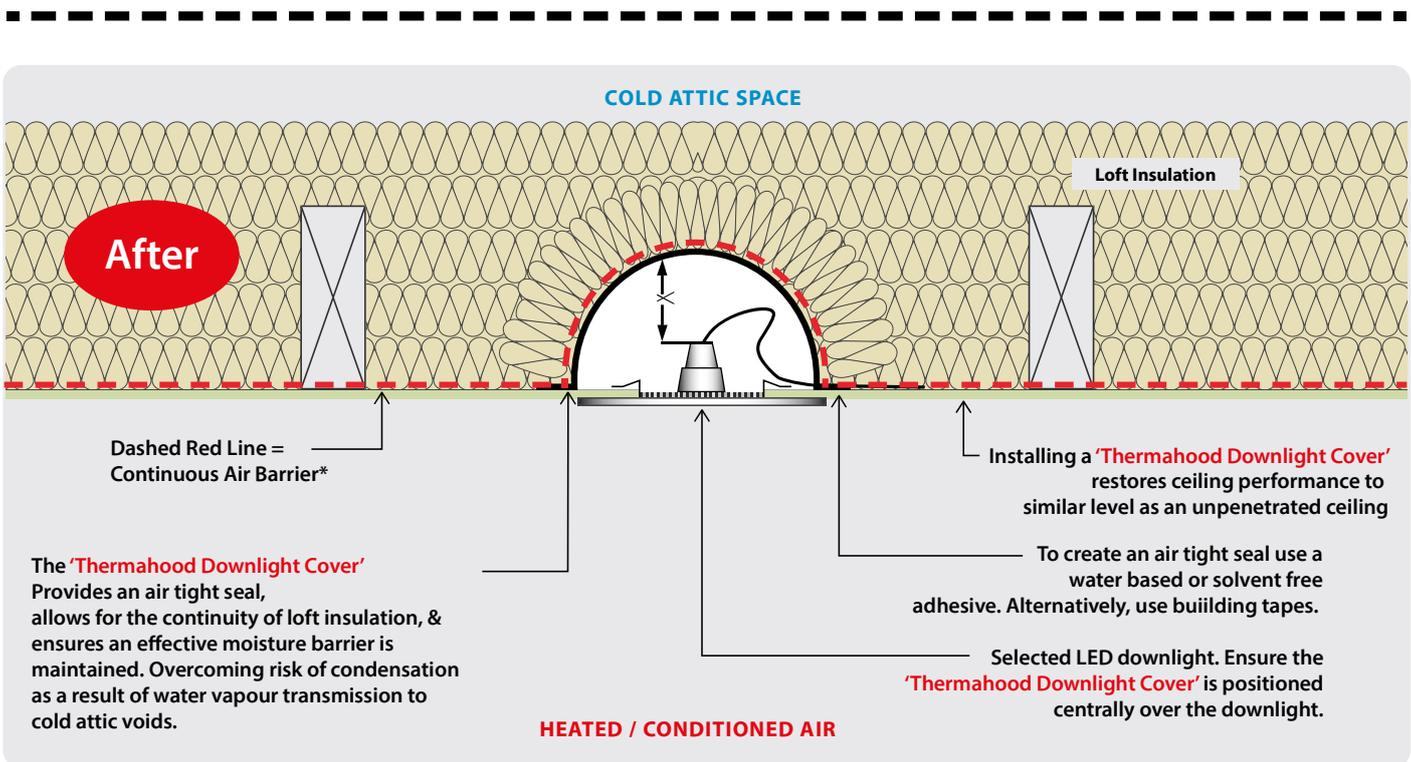
Thermahood helps guarantee building standards for professional builders by minimising the risks involved in installing unprotected downlights. **Loft or attic insulation effectiveness can be improved by as much as 50% by using Thermahood Downlight Covers!**
