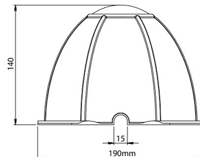
**TH 001** is the most popular product in the Thermahood range as it can be easily fitted over most downlights. Squared sides allows for fitting close to joist and there are four corner flanges for fixing in position.
