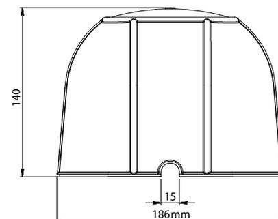
**TH 140** has more space inside due to the square shape and has no flange, this allows for fitting close to joist or rafters. TH 140 can be used with larger downlights and with downlights which have the connector block fixed at 90 degrees to the light fitting.
