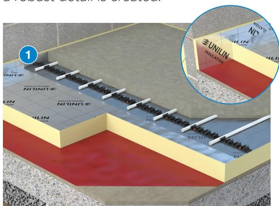
2. Thin-R Underfloor is lightweight and suitable for use with underfloor heating. Thanks to its thickness to performance ratio, it allows for reduced insulation thickness. The boards should be laid with closely butted joints, laid staggered with a break bonded pattern and fitted tightly at edges and around any service penetrations.
