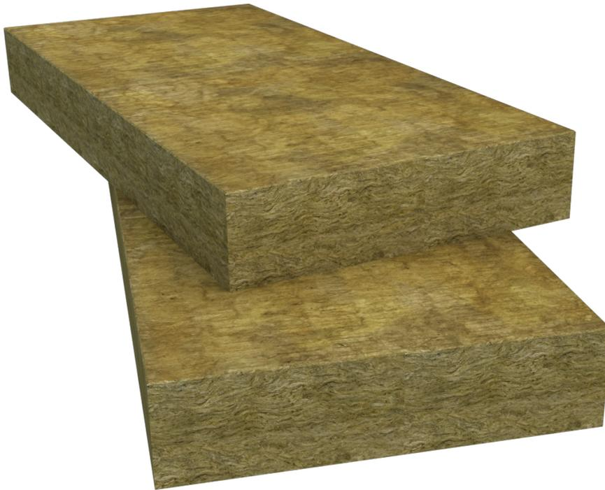
When building with timber, using non-combustible ROCKWOOL insulation can help to reduce the risk of fire, and fire spread, particularly during the more vulnerable construction phase. Tested to BS EN 13501-1, achieving the highest possible Euroclass reaction to fire classification of A1, Timber Frame Slab acts as a barrier to fire, able to withstand temperatures over 1,000°C.
