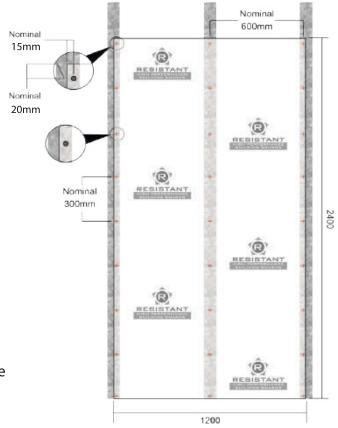
When fixing to receive render, boards should always be fitted with stainless steel screws.
